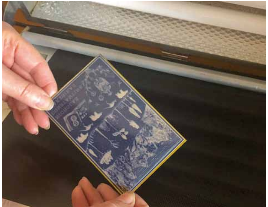
Exposing the photopolymer plate through the negative
